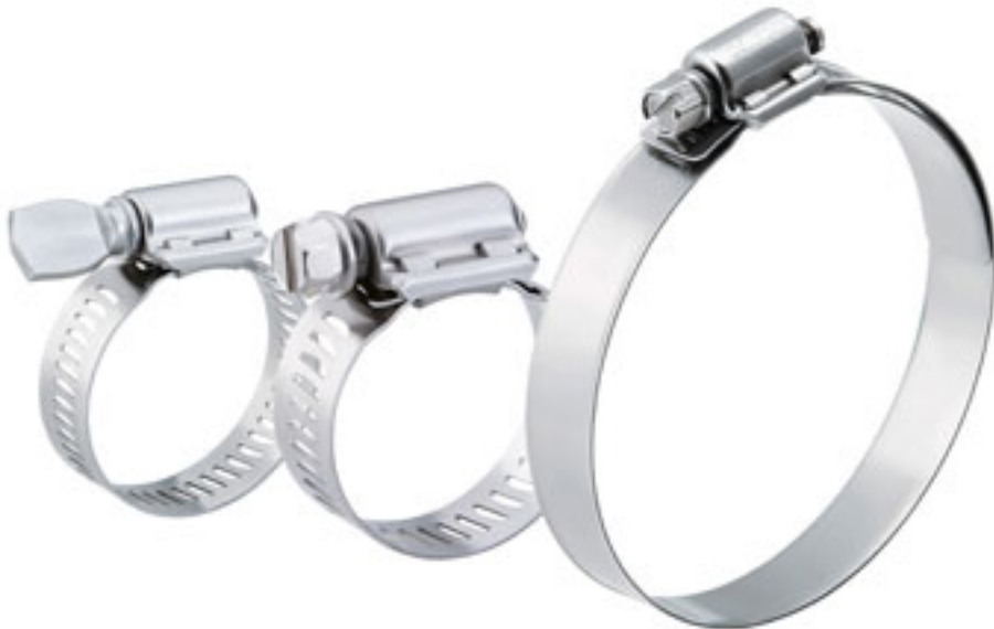
Aviation Worm Drive Hose Clamp We offer a variety of hose clamps engineered specifically for the aviation industry. The clamps are exceptionally light due to the perforated band. The thread is engineered to be vibration proof and easy to install when needed. Optional with hole for locking wire.
